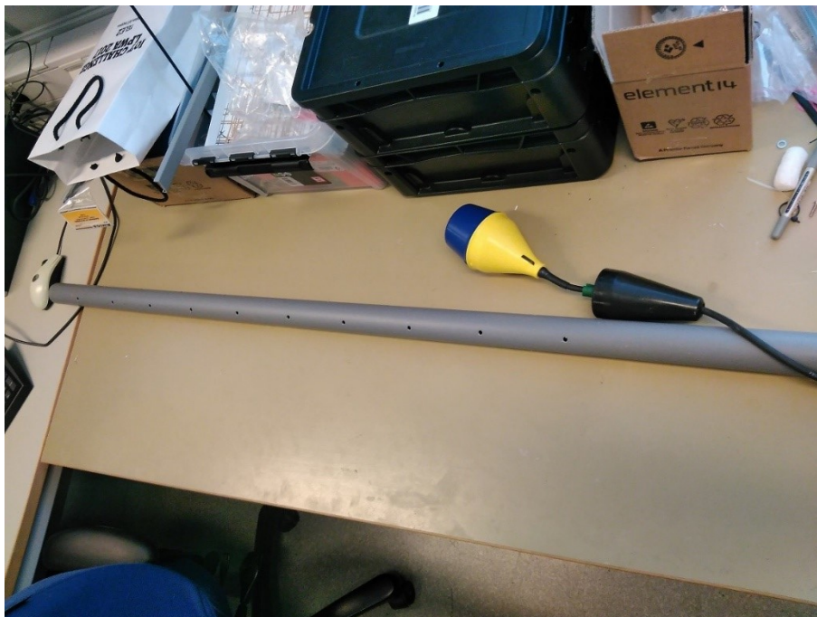
Figure 13: Hydrostatic sensor in the tube and floating switch outside, plus LoRa control and communication box. Image courtesy of Dimitar Kolev, RISE AB
