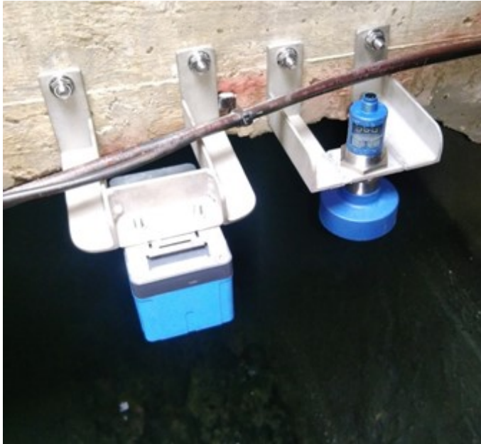
Figure 9. Radar sensor (fully equipped with radar, battery, GSM 2G communication, GPS, Bluetooth) and Ultrasonic sensor (cable not attached). Both sensors are non-contact ones, so no garbage collection and no maintenance are needed. Image courtesy by Dimitar Kolev, RISE AB.
