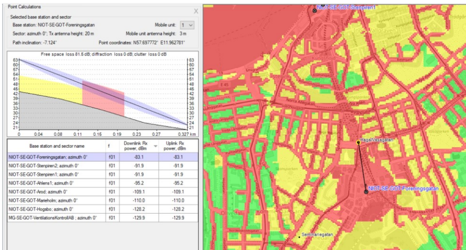
Figure 5: Calculated signal strength at street level, by manhole in Haga/Vasagatan.
